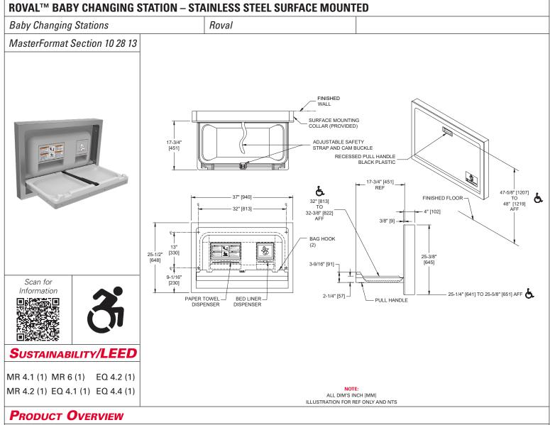
ADA-compliant unit features welded stainless steel for long and reliable use. Exposed surfaces are satin finish. Easy onehanded operation is assisted by a pull handle and concealed spring. The changing surface is high-impact-resistant plastic for easy cleaning. Its two part adjustable safety strap and 50 lbs (23 kg) load capacity assure child protection. Tested during development to sustain 300 lbs (136 kg) static load with minimal deflection. Surface mounted with stainless steel collar.
